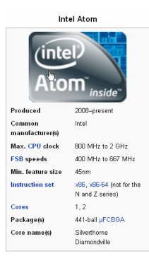
**Intel Atom** is the brand name for a line of x86 and x86-64 CPUs (or microprocessors) from Intel, designed in 45 nm CMOS and used mainly in Netbooks. The Atom Z series is code-named Silverthorne and the Atom N series is code-named Diamondville. As of June 2009, the most used chips in the Netbook retail market are Z520, Z530, and N270.
