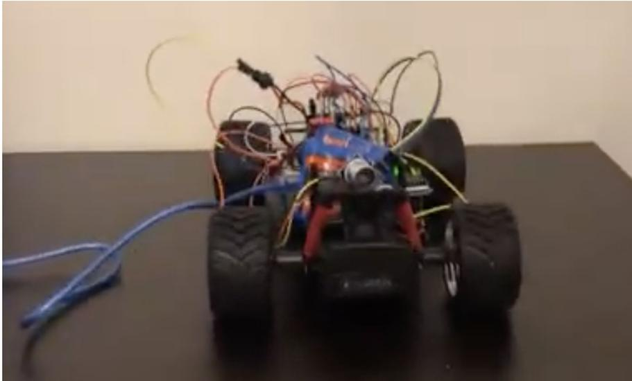
We then moved on to use a design in which the raspberry pi controls the movement of the car along with the electronic speed controller and the servo shield. The arduino was used mainly for collecting sensor data from the ultrasonic sensors, which is then passed on to the raspberry pi. To power all the components, a power bank was used to power the raspberry pi and arduino and the LiPo battery used to power the ESCs.
