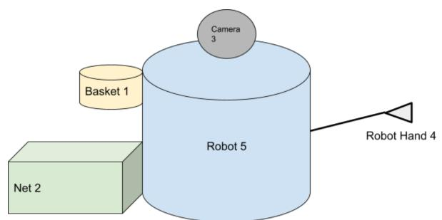
The on board camera 3 based sensor scans the debris and determines if it should be stored in the attached basket 1 (for smaller items) or net (for larger items) 2. The robot has a net 2 and basket 1 connected to it and a robot hand 4 that will grab debris and place it in the attached net 2/basket 1.
