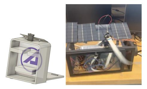
The final design consists of a chassis that holds the satellites with the camera, motors, and lasers attached to the Jetson Nano and Arduino.
