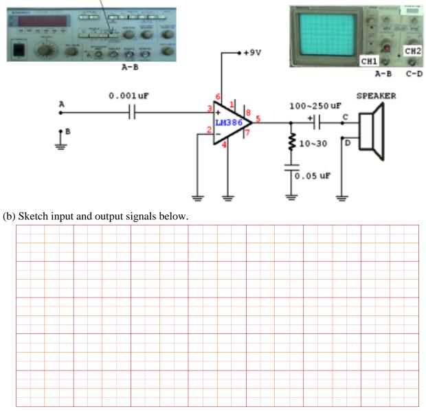
(c) Change the frequency of the sinusoidal signal to 200Hz, 1000Hz, and 2000Hz, and describe the sounds from the speaker.
