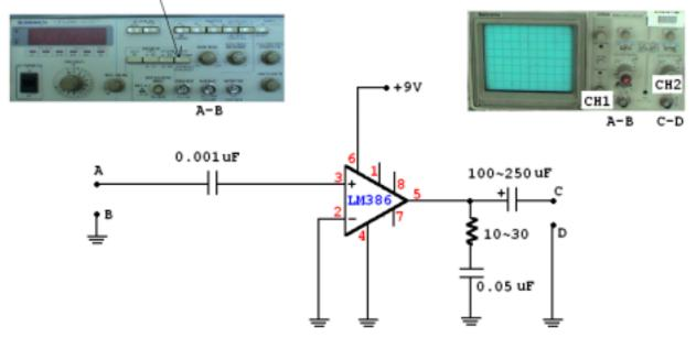
(c) Sketch input and output signals below. And find the **gain** of Output/Input.
