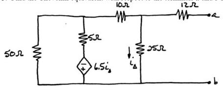
4. Find the Thevenin equivalent with respect to the terminals *a* and *b* for the circuit below.
