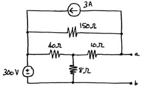
2. Find the Thevenin equivalent with respect to the terminals *a* and *b* for the circuit below.
