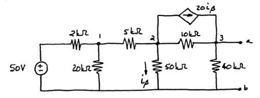
3. Find the Thevenin equivalent with respect to the terminals *a* and *b* for the circuit below.
