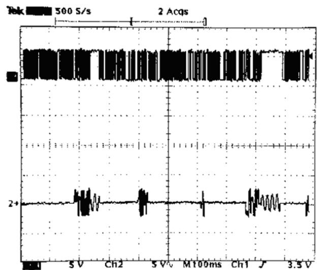
Fig.5. The generated bit stream (upper trace) from the TX and the disrupted carrier signal over the wire (lower trace) caused by rubbing spike noises [17].
