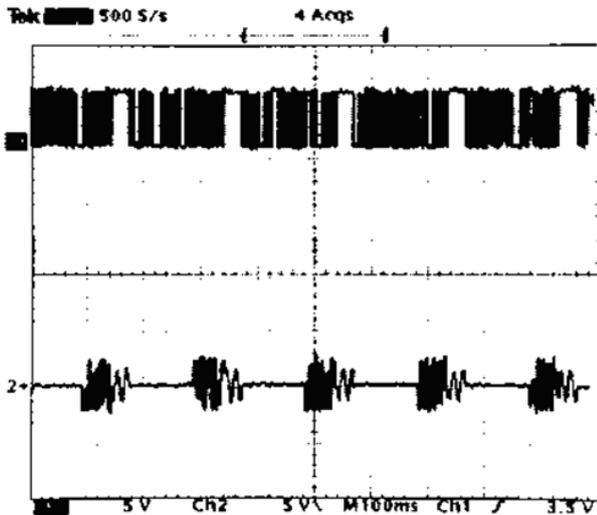
Fig.3. Digital bit stream generated by TX (upper trace) and its FSK modulated carrier signal over the wire (lower trace) [17].
