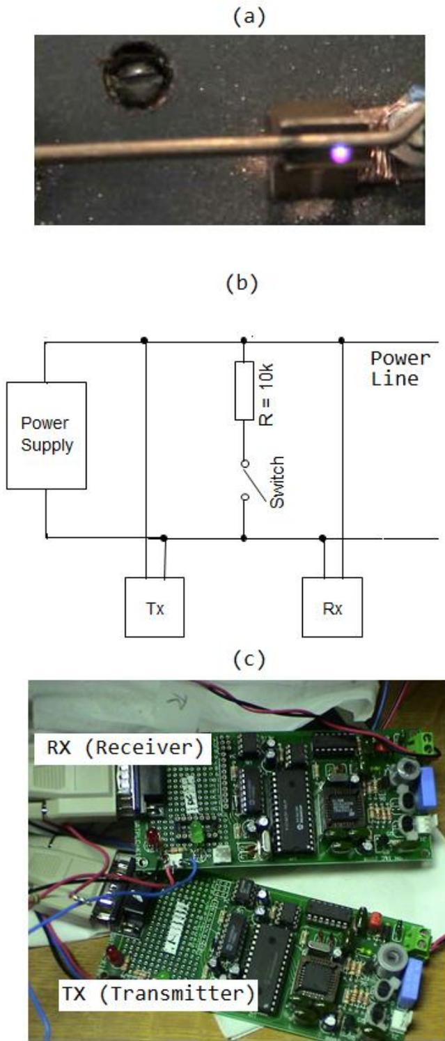
Fig.1. PLC transceiver prototypes and experiment setup with a knife switch to simulate intermittent wire contact with foreign object. (a) vertical arcing from the knife switch, (b) experiment setup configuration diagram, and (c) PLC transceivers.
