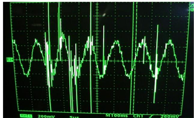
Fig. 2. The impulse spikes generated by knife switch rubbing disrupting the sinusoidal PLC signal transmitted in the wire.
