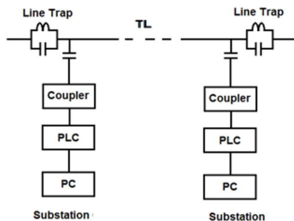
Fig. 7. A proposed PLC configuration for transmission line monitoring for vegetation or foreign object contact.
