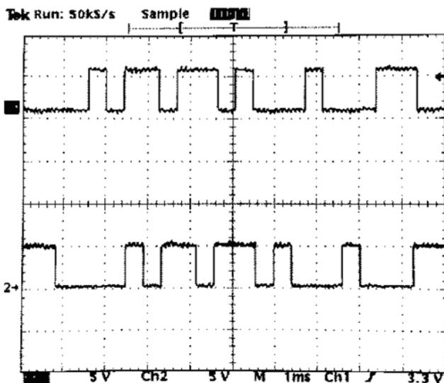
Fig.4. The same digital bit stream of TX (upper trace) and RX (lower trace) sides under normal condition [17].
