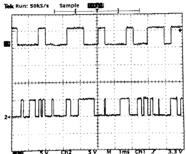
Fig.6. The difference between the transmitted digital bit stream (upper trace) and the received (lower trace) under a fault condition [17].
