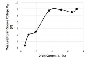
Fig. 7. Measured (dots) points for V<sub>DS</sub> magnitude for varying I<sub>D</sub>
