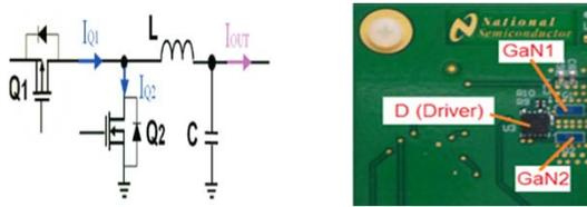
Fig.1. Circuit Diagram (left) and a part of PCB (right) of LM5113 Evaluation Board.
