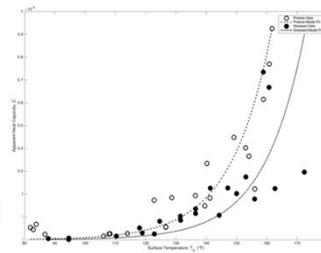
Fig. 5. Apparent heat capacity C<sub>A</sub> vs surface temperature, T<sub>s</sub> data for pristine and stressed GaN FETs with an exponential fit
