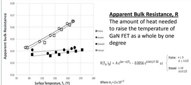
Fig. 4. Apparent bulk resistance vs. surface temperature of GaN FET for pristine and stressed GaNs in two separate set of experiments
