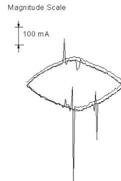
Fig. 4. Leakage impulse current on elliptical time base.
