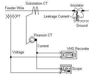
Fig. 2. Leakage impulse data-acquisition setup.
