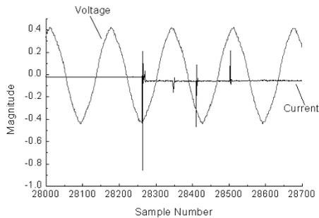
Fig. 3. Sinusoidal voltage and leakage current waveform.
