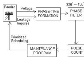
Fig. 9. Illustration of the insulator status monitoring.
