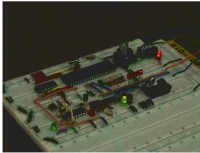
Fig. 102 Implementation of IR Master on breadboard
