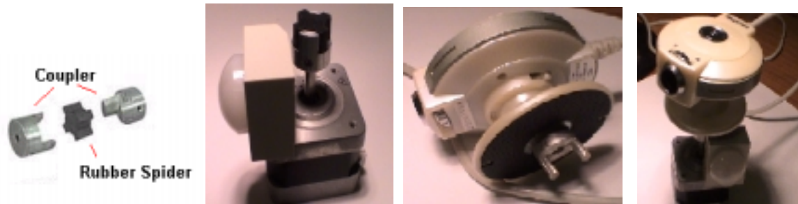
Fig. 52 Few different sets of couplers for different shaft diameters
