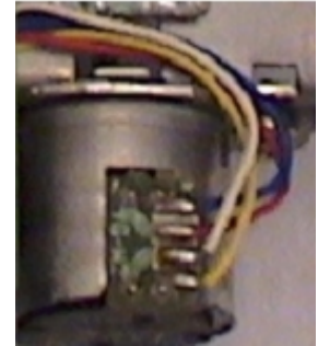
Fig. 49(c) 12 V head motor inside a floppy disk driver
