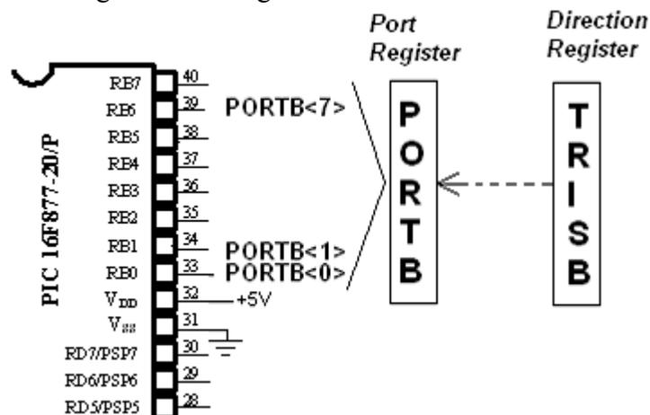
Fig 5. Port register and corresponding direction register
