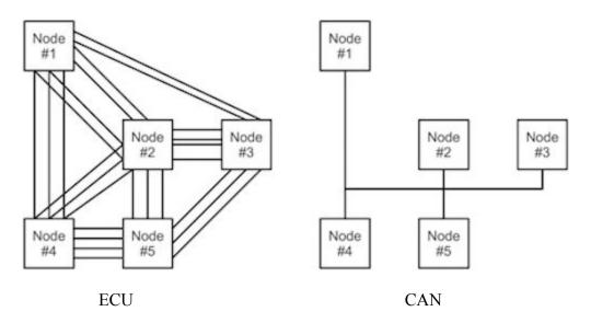
Before the CAN bus network, the engine control unit(ECU) was the main source connecting everything micro controllers to devices in the car. Reason there were many wires. But the CAN bus dramatically reduce the amount of wires used.
