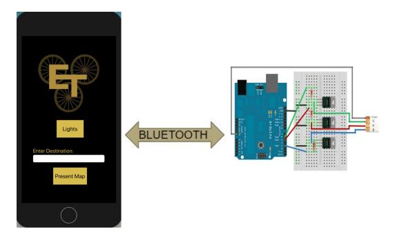
Each "buttonTapped" function above correlated to a different light which was signified by a different hexadecimal input. Orange was 0x31, red was 0x32, white was 0x33, and off ws 0x30 in the swift code. In the Bluetooth code for arduino, these inputs equated to 1, 2, 3 and 0 respectively as shown below.
