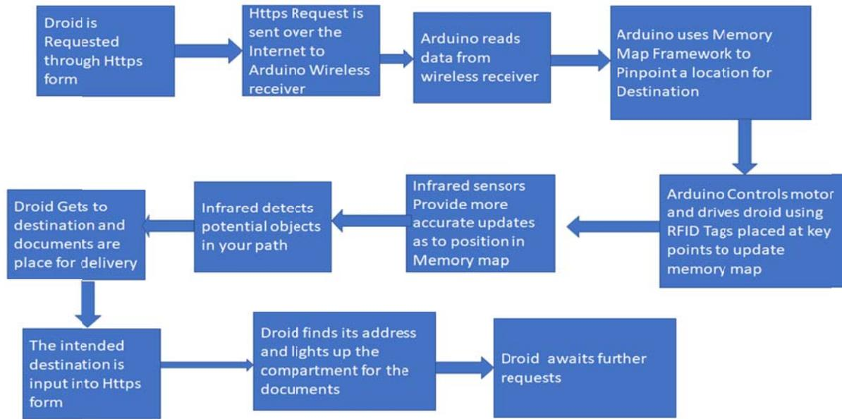
This diagram depicts the process by which the robot will potentially be interfaced with by a user and how it uses the information to go to a specific loading point and then find its way to the intended destination. It is all done through the internet which means it requires a simple web server to process input data from users.
