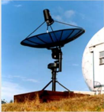
MIT Haystack SRT specifies the use of a 90 inch antenna with a beam width of 7.0 degrees. We conducted further research on how to determine the beam width, or angular resolution, of an antenna. The angular resolution ( $\theta$ ) of a telescope defines its ability to distinguish specific details in an image. The smaller value of  $\theta$ , the better the resolution the telescope will have.
