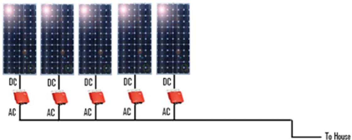
Figure 1 micro inverter conceptual design
