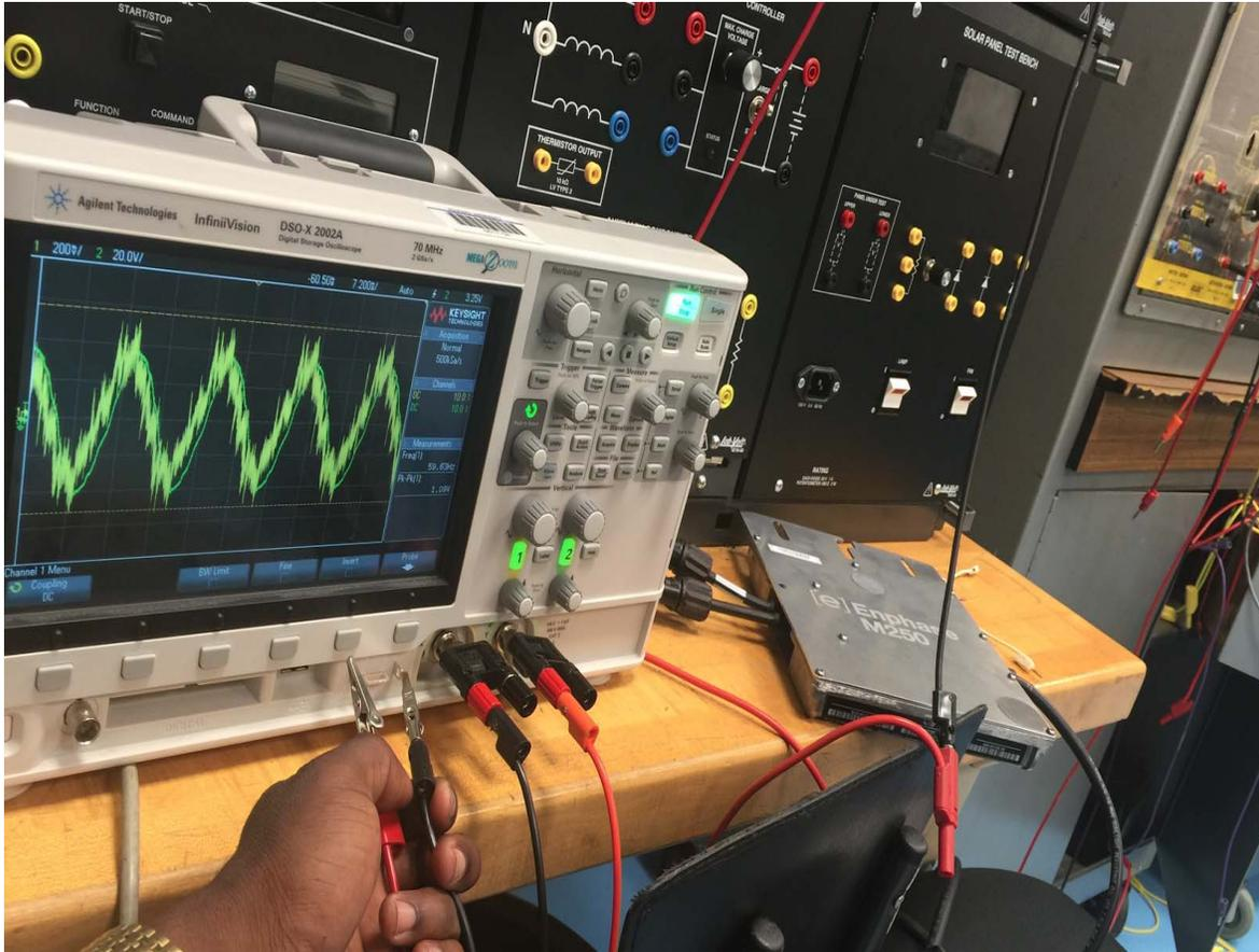
Figure 5 Testing for the output AC signal from two micro inverter connected in parallel
