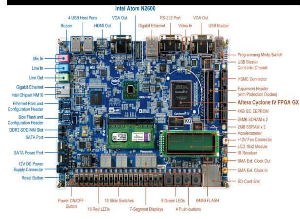
The final design will use the intel de2i-150 board. This board has an LCD screen equipt. The tablet's size will be roughly the size of this board. A usb camera, micro SD storage wil be the peripherals added.
