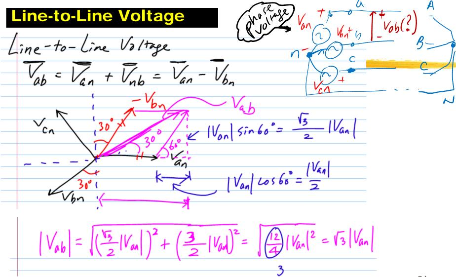
$$|V_{ab}| = \left(\frac{\sqrt{5}}{2}|V_{an}|\right)^{2} + \left(\frac{3}{2}|V_{an}|\right)^{2} = \left(\frac{12}{4}|V_{an}|^{2} = \sqrt{3}|V_{an}|\right)^{2}$$
