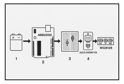
The Glow Garments system is powered by a 5V rechargeable battery [1], which supplies voltage to the Arduino Uno microcontroller [2], a compact breadboard [3], and the WS2812B LED strip [5]. The Arduino [2] controls the lighting logic and is programmed to respond to motion input from the MPU6050 accelerometer [4], which is mounted on the breadboard [3]. The breadboard [3] serves as the central wiring hub, distributing power from the battery [1] to the accelerometer
