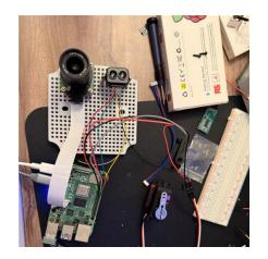
File Edit Taba H&P Site distance: Distance: 142.00 cm | Strength: 2958 | Temp: 49.00°C Safe distance. Distance: 222.00 cm | Strength: 2463 | Temp: 49.00°C Safe distance. Distance: 80.00 cm | Strength: 2094 | Temp: 49.00°C \*\*\* Object within critical distance! Week 3: Have portable battery power the system, mount sensing system to protective casing
