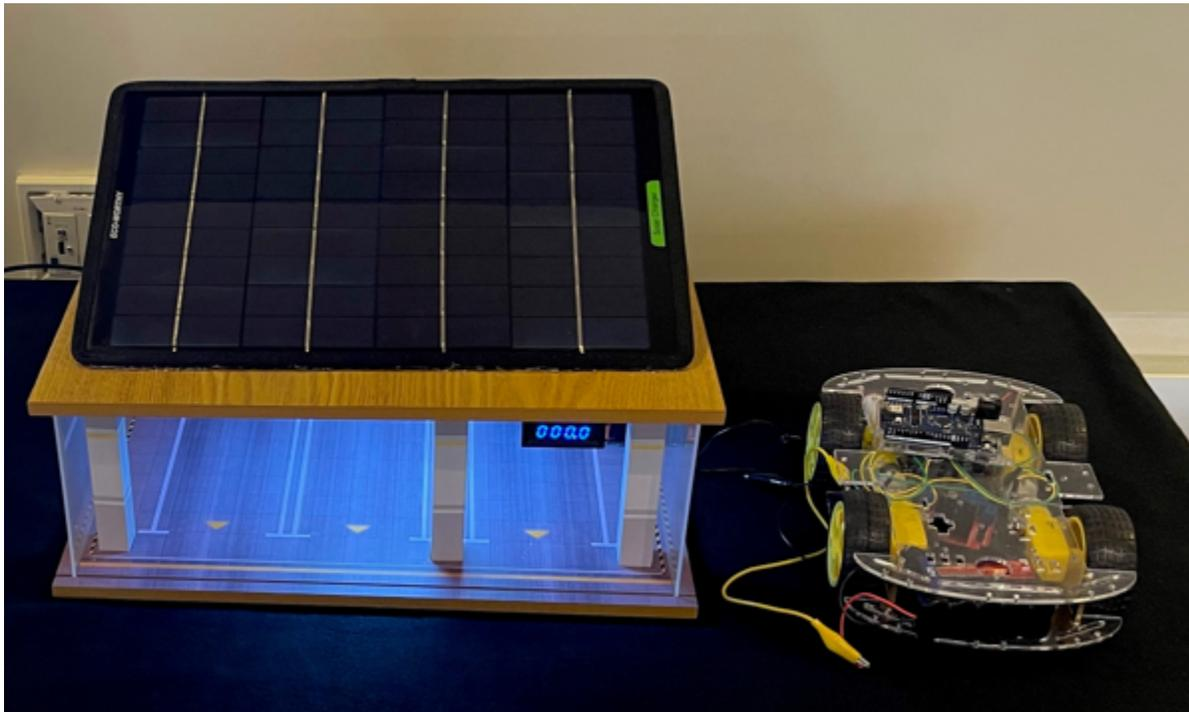
Pictured above is the completed charging station with the vehicle attached. The solar panel is placed on top of the charging station which houses the charge controller and an additional battery (both not pictured). The digital display is that of a voltmeter. The vehicle contains the motor driver and battery on a lower level and the arduino on the top level. As discussed in the solution design, four dc motors control the movement of the vehicle.
