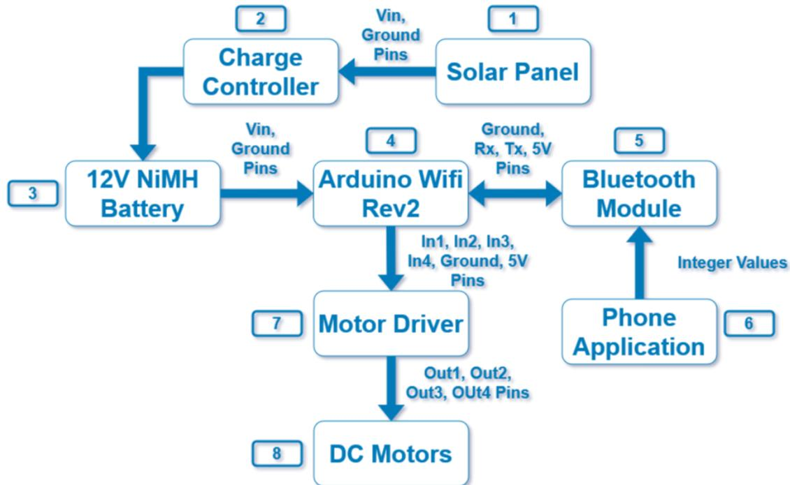
1. The solar panel included on this project is a 10W 12V device connected to the charge controller. This panel was placed on top of the structure built to house and store the vehicle. The angle chosen was based on what would be the most efficient year round on our campus.
