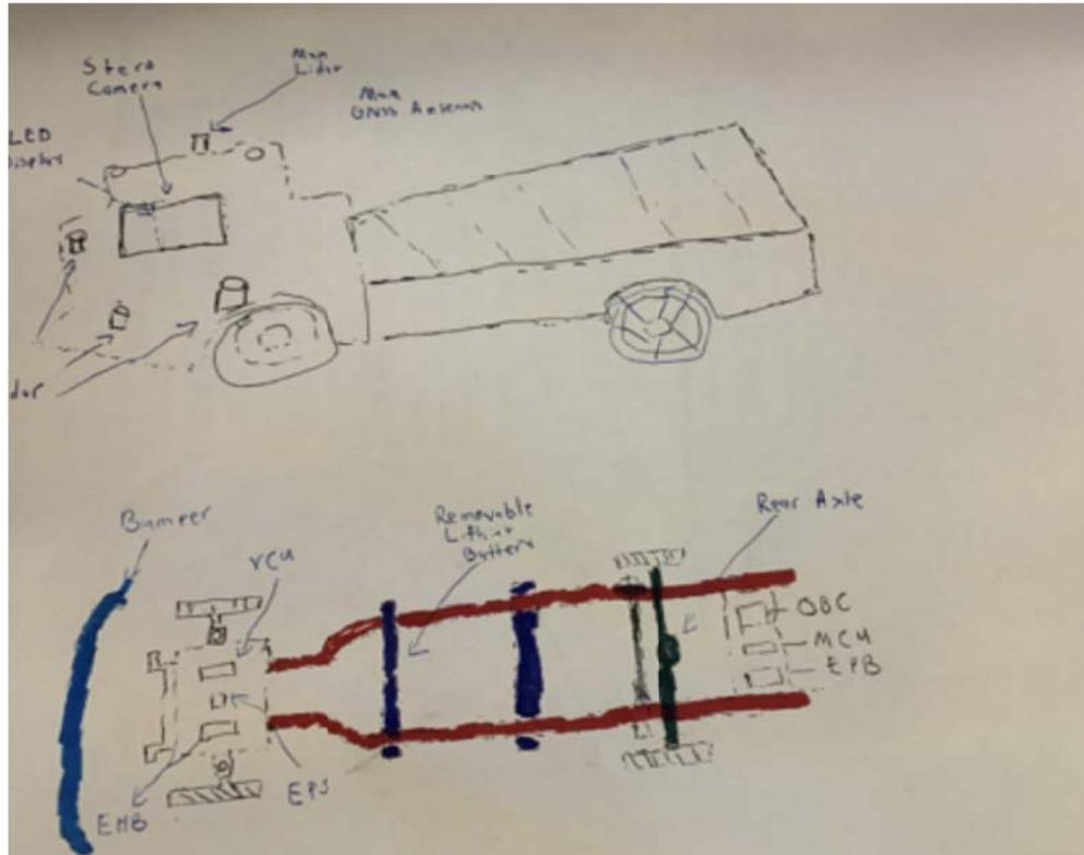
This design will follow a design layout similar to a pickup truck. The idea is to have a truck bed that will hold the documents that we want the device to transport. The size of this device will be much larger than that of the Small Truck design, and this will allow for users to load larger and heavier documents to the device that the Small Truck would not have been able to.
